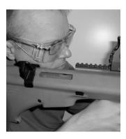
2 o'clock to 3 o'clock direction approximately 3 to 15 feet from the rifle in a slight upward arc. Test 10 more rounds on the "H" or "High" gas setting. The ejection should be similar or a few feet farther.
