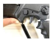
slightly to help it find the "sweet spot" and seat. Screw the grip back in solidly with the 5mm allen wrench.
