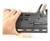
Push the long bolt in. If you meet resistance press down on the bolt and wiggle it a bit. You can also try inserting from the other side. A small hammer with light taps can help the bolt through the hole in the rail. Once through, thread the second bolt into the first.
